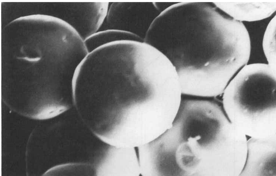
FIG. 7. SEM photograph of salicylaldehyde-acrylate-divinylbenzene copolymer.
